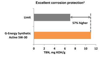
Extended TBN reserve to neutralize acidic by-products of combustion for higher corrosion protection helps to extend overhaul intervals
